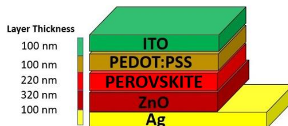
Fig. 16. Simulated Perovskite Solar cell with layer Thickness
