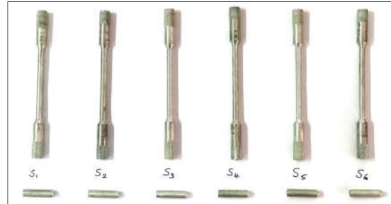
Fig. 3. Tensile and wear test samples
