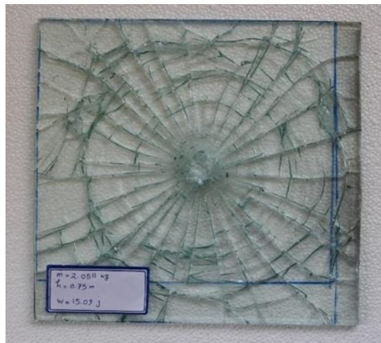
Fig12. .specimen after test code D-B-T-5
